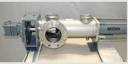
The two inspection openings which have been incorporated above the joints of the coupling rod are the greatest difference with respect to conventional systems. These mean that it is possible to check whether the joints are still sufficiently lubricated and the seals are still intact while the pump is in operation.
