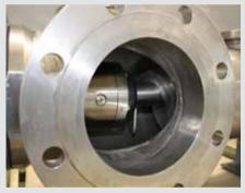
These geared joints are different from pin joints; they have a double seal to provide increased safety. If one of the rubber sleeves becomes cracked, the second one beneath automatically maintains the seal.
