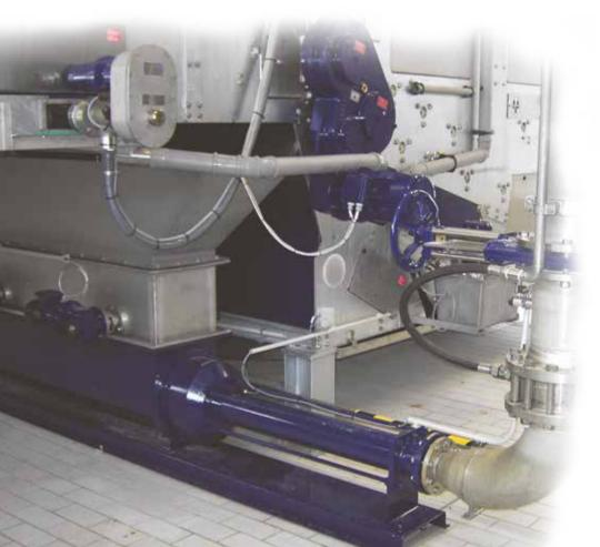
NEMO<sup>®</sup> Sludge Cake Pump with customized 4.27 ft / 1.5 m hopper pumping 20 - 22% dewatered sludge from a belt filter press to a drying plant 110 ft. (34 m) away. Pump employs dual aBP-Module<sup>®</sup> (Asynchronous Bridge Preventing Module), STP stator dry running protection system and the Friction Loss Reduction System (FLR - see page 8 and 9).
