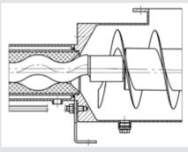
NETZSCH's patented positioned feed screw
