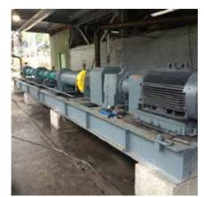
Slurry pump for coal mine in USA
